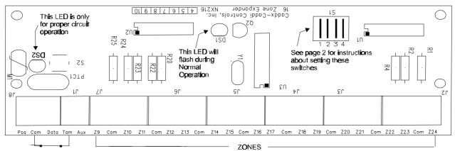
Pos, Com, and Data - Connect to keypad terminals on the NX-8 or the NX-320. Tam - Connect to Com terminal through a normally closed switch.
