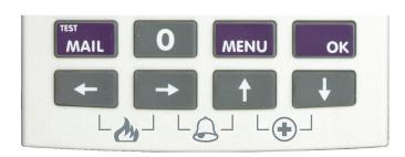
Figure 42: Keypad Emergency Keys
