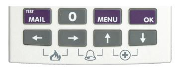
Figure 8: Keypad Emergency Keys
